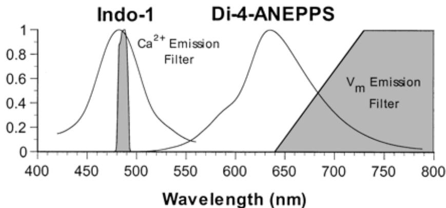
**Fig. 2.** Normalized transmittance characteristics of emission filters (gray area) selected for indo 1 ( $\text{Ca}^{2+}$  emission filter,  $485 \pm 5$  nm) and di-4-ANEPPS [membrane potential ( $V_m$ ) emission filter,  $>695$  nm] superimposed on normalized emission spectra (solid lines) of indo 1 (excitation 365 nm) and di-4-ANEPPS (excitation 515 nm). On the basis of the emission spectra, filters were chosen to minimize spectral overlap and maximize signal strength.
